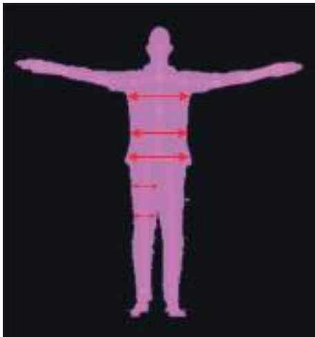
FIGURE 5: Background removed body index image with front horizontal curve in depth space.
