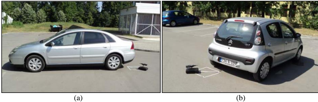
Figure 4- Position of cars at the test site and the microphone position
