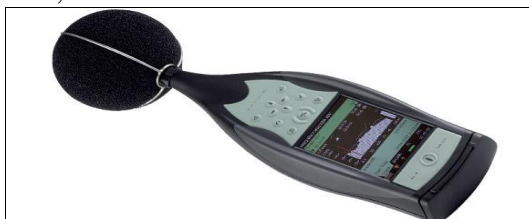
Figure 3- Sound level Meter type 2250 produced by Bruel & Kjaer
