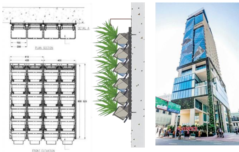
Figure 3: Living wall system details in the Sri Lankan market and Movenpick hotel (Wall Span, 2017)
