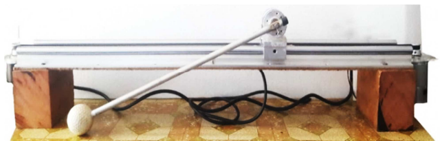
Figure 4. Inverted Pendulum after construction.
