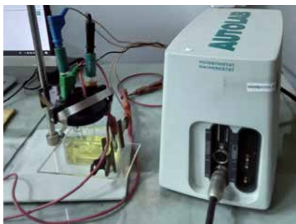
EIS analysis using potentiostat
